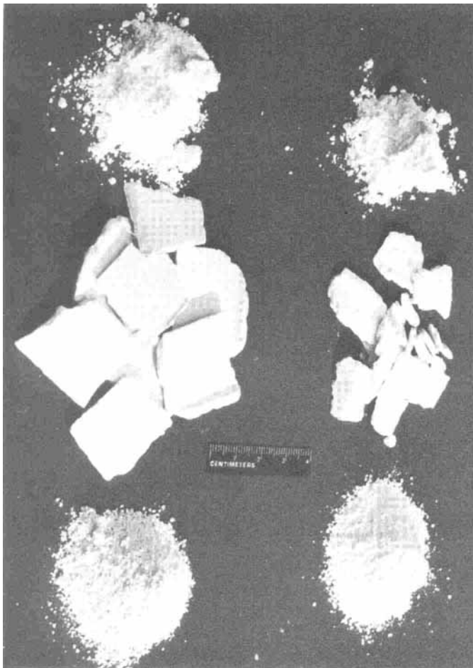
Figure 3 —Bulk and roller compacted materials. The upper piles are the bulk powders, the middle samples are the flakes of compacted materials, and the lower piles are the compacted granules prepared by passing the flakes through a 1.0-mm screen in an oscillating granulator. Aminobenzoic acid is on the left, and sulfadiazine is on the right.
